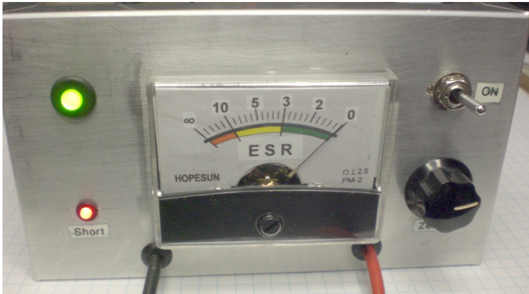
Zero Meter, note that Short LED is On
